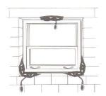
2. Installing Windows & Doors – The Universal Air Wedge™ holds windows and doors in place while leveling for easier installation. Simply slide the Universal Air Wedges™ around window or door and inflate.
