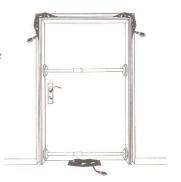
**3. Holding Doors Open** – The Universal Air Wedge<sup>™</sup> is an inflatable door stop that holds doors still during lock installation. When the door is open, slide the wedge underneath the door.
