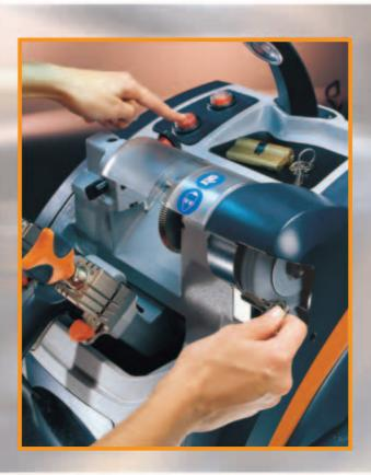
Karat is provided with a micrometric adjustment of the tracer enabling the user to apply a precise set up or correction of the cutting depth especially in the case of worn out keys.
