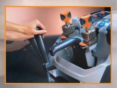
The carriage is equipped with security devices purposely designed for a safe, easy and interactive release and control functions of the gauge position avoiding accidental start up of the cutter.
