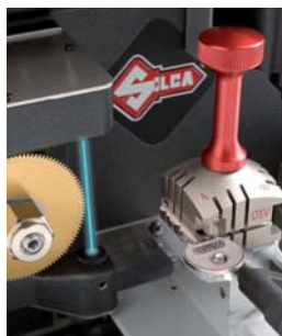
Prismatic cutter and optical reader for flat keys
